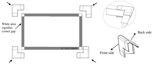
Once all corner sleeves have been snapped into each corner of the frame, it is ready to be installed.
