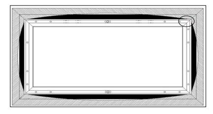
Pull back the screen material from the velcro connection along the edges of the frame to detach it.
