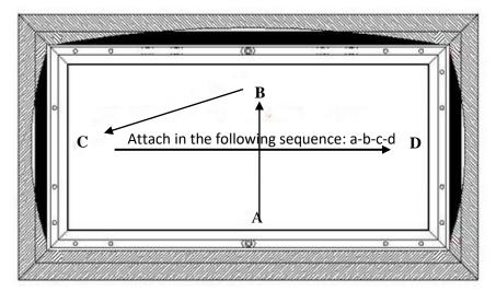
6. If the material is too loose or tight after adjusting all four corner sides, then you will need to reattach the material.
