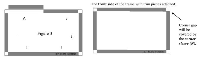
4. After the bezel trim has been installed, place a *corner sleeve (M)* on all four corners. Begin by aligning and adjusting the corner sleeve through the front of the screen. Make sure the corner sleeve completely wraps the edge of the bezel trim. This should cover any corner gaps.
