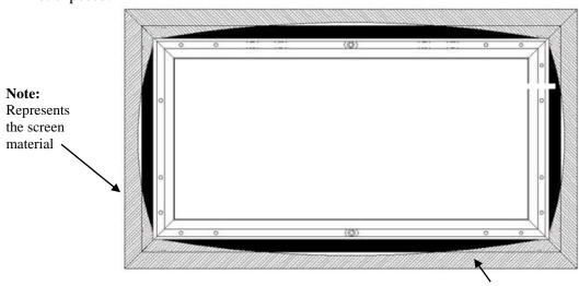
**Note**: The black shaded part represents the velcro on the frame. That Velcro end will ultimately attach with the other velcro end on the screen material.
