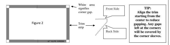
**NOTE:** Make sure the bottom edge trim with the Elite Screens logo is installed on the correct side. The back of the material should be labeled with a DOWN sticker to indicate the material is facing in the down position. The Elite Screens logo should be installed on the DOWN side
