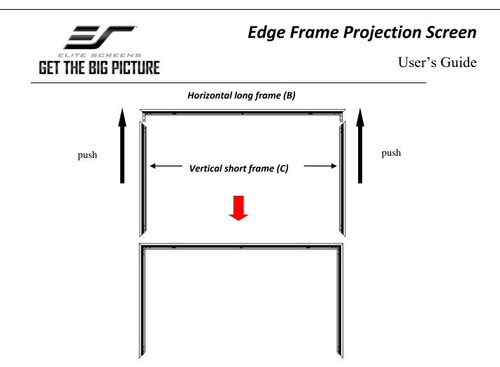
6. Join the remaining *horizontal long frame (B)* with the frame built in the previous steps as shown below.
