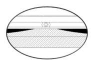
Lay the Velcro end on the screen material over the Velcro end of the frame and keep it within the edge.
