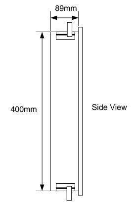
Minimum Wall Thickness: 9mm Maximum Wall Thickness: 60mm
